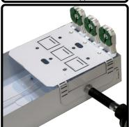
GREEN sockets are wired to NEUTRAL. Install the socket bar with GREEN sockets at the opposite end of the fixture using the #8 Tek screws provided.
