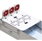
**RED** sockets are wired to **LINE** voltage. Install the socket bar with RED sockets at one end of the fixture using the #8 Tek screws provided
